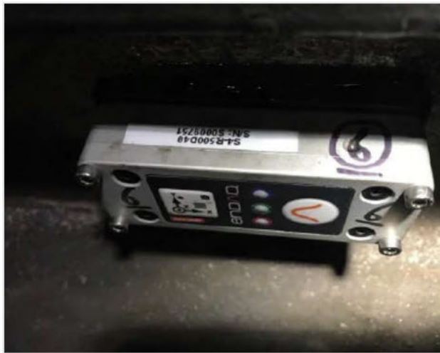
Figure 11: Stock rail fitted enDAQ Sensor
